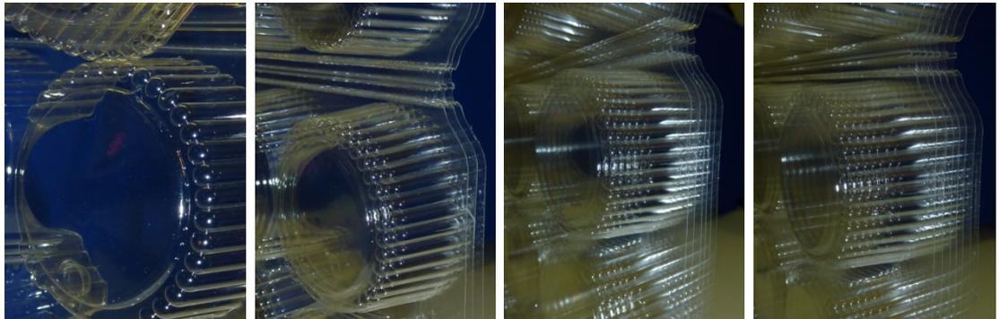
in connection with an **A-LAS-CON1** control electronic is used. At this a part of the laser beam will be reflected and absorbed, as more blister packages are present as higher is the reduction of the laser beam. The screenshots shows the decrease of the signal dependent of the number of blisters.
