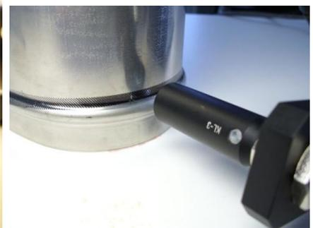
the metal surface. Even a color shift can be observed. The distance from the optical front end to the object is around 11mm and the spot size is approximately 1mm (diameter) or 4x0.7mm<sup>2</sup>.
