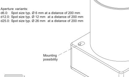
Receiver optics incl. 3-color filter detector (True Color), transmitter optics with white light LED (scratch-resistant optics cover made of glass)
